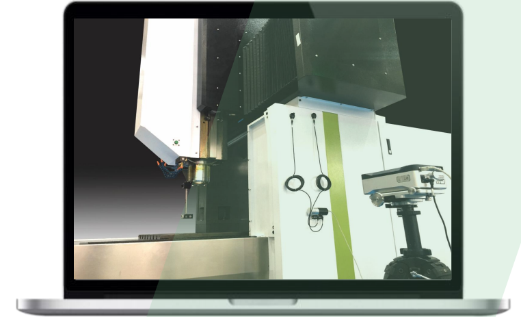
Laser interferometer positioning accuracy inspection
