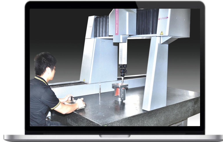
Japan Mitutoyo 3D parts accuracy inspection
