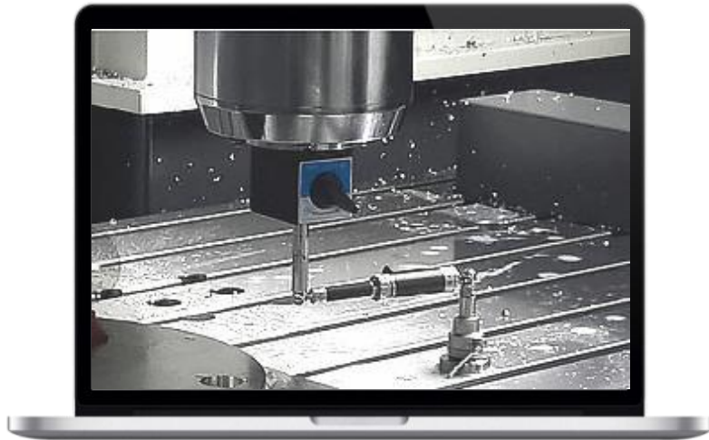
Renishaw Ballbar Circularity inspection
