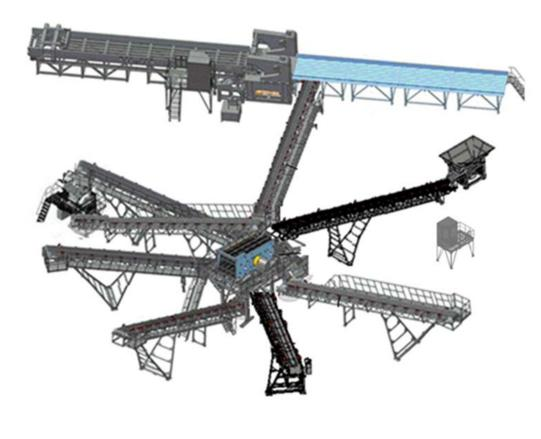
technological The line of includes complex a assemblies and mechanisms for preliminary recycling of dismantled products, the production defects of plants manufacturing reinforced concrete products as well as construction waste, etc. with subsequent automatic separation of reinforcing bars and metal inclusions, crushing and sorting in order to obtain secondary crushed stone of the necessary fractions.
