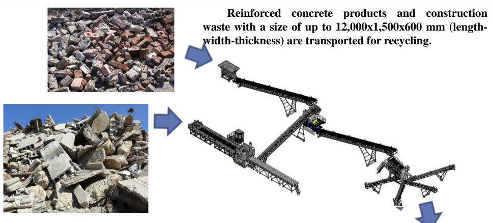
Downstream the MPR-1500 recycling complex, there the following fractions of the classified ready-building material (crushed stone): 0– 5 mm, 5–20 mm, 20–40 mm, 40–70 mm; reinforcing wires/bars fit for scrap. The performance of MPR-1500 is up to 100 ton/h, the power consumption of the complex-up to 180 kW.
