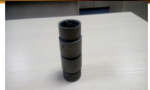
Crashworthy aggregates made with the help of additive technology(3d print)
