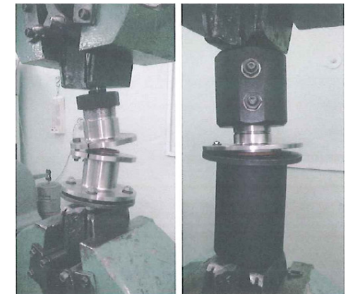
valve after durability test under the action of axial load
