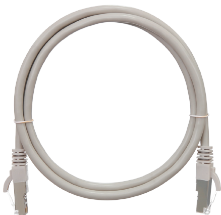
NMC-PC4SD55B-XXX-C-GY - LSZH NMC-PC4SD55B-XXX-GY - PVC F/UTP, Cat.5e, RJ45-RJ45
