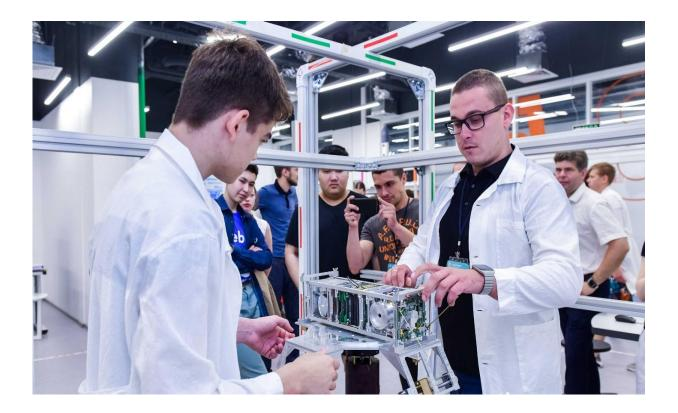
The purpose of using the test bench is experimental testing and research of the operation of the orientation, stabilization and navigation algorithms of the spacecraft in terrestrial conditions.
