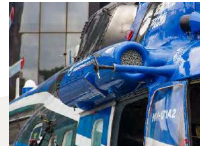
air conditioner / heater
