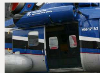
right widened door
